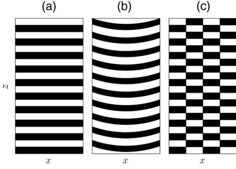
Fig. 1. Diagram of three QPM structures: (a) standard, (b) parabolic, and (c) with multiple dislocations.
