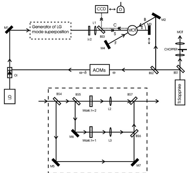
Fig. 2. Experimental setup: OI, optical isolator; BS1–BS7, beam splitters; M1–M7, mirrors; L1–L3, lenses; MOT, magneto-optic trap;  $\lambda/2$ , half-wave plate; D, detector; LD, laser diode. Other terms defined in text. Inset, double Mach-Zehnder interferometer to generate different superpositions of LG modes.
