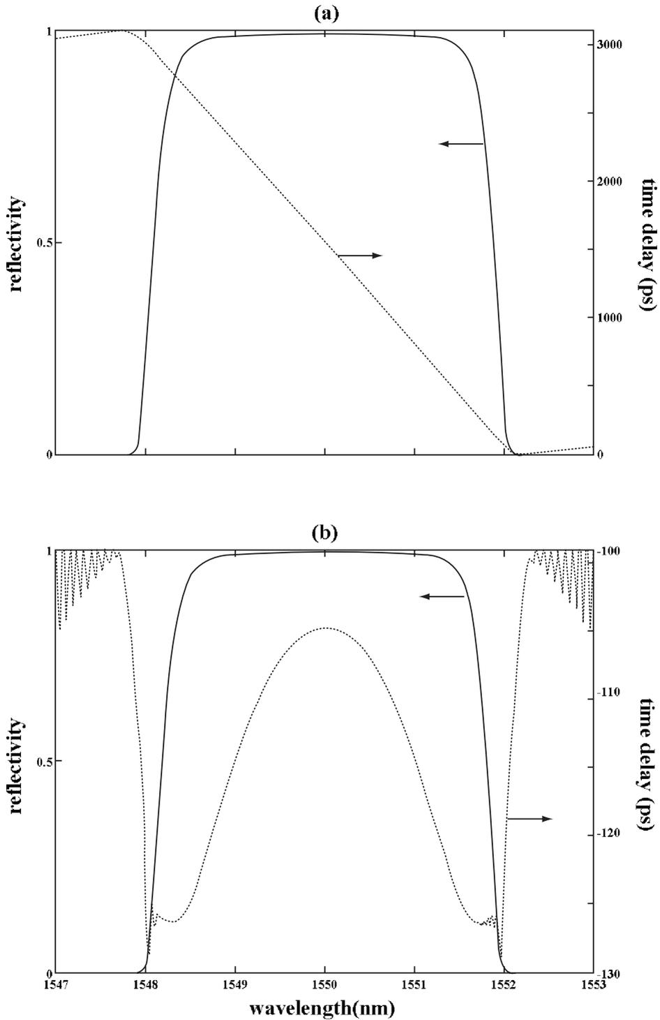
Figure 2. Reflectivity and group delay of the FBG used for dispersion compensation slope with measure of the sharpness  $a = 4$ . (a) Response of each individual grating and (b) response of two combined FBG with opposite chirp.
