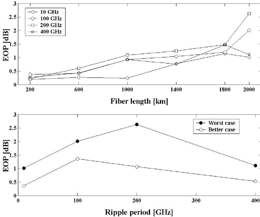
Figure 4. Worst eye opening penalty in dB for different periods of the ripple with  $A_{\text{GDR}}=1$  ps at different fibre length. In the lower picture, better and worst cases are represented for 2000 km. Five simulations for each period are considered. The solid line is to help the eye.
