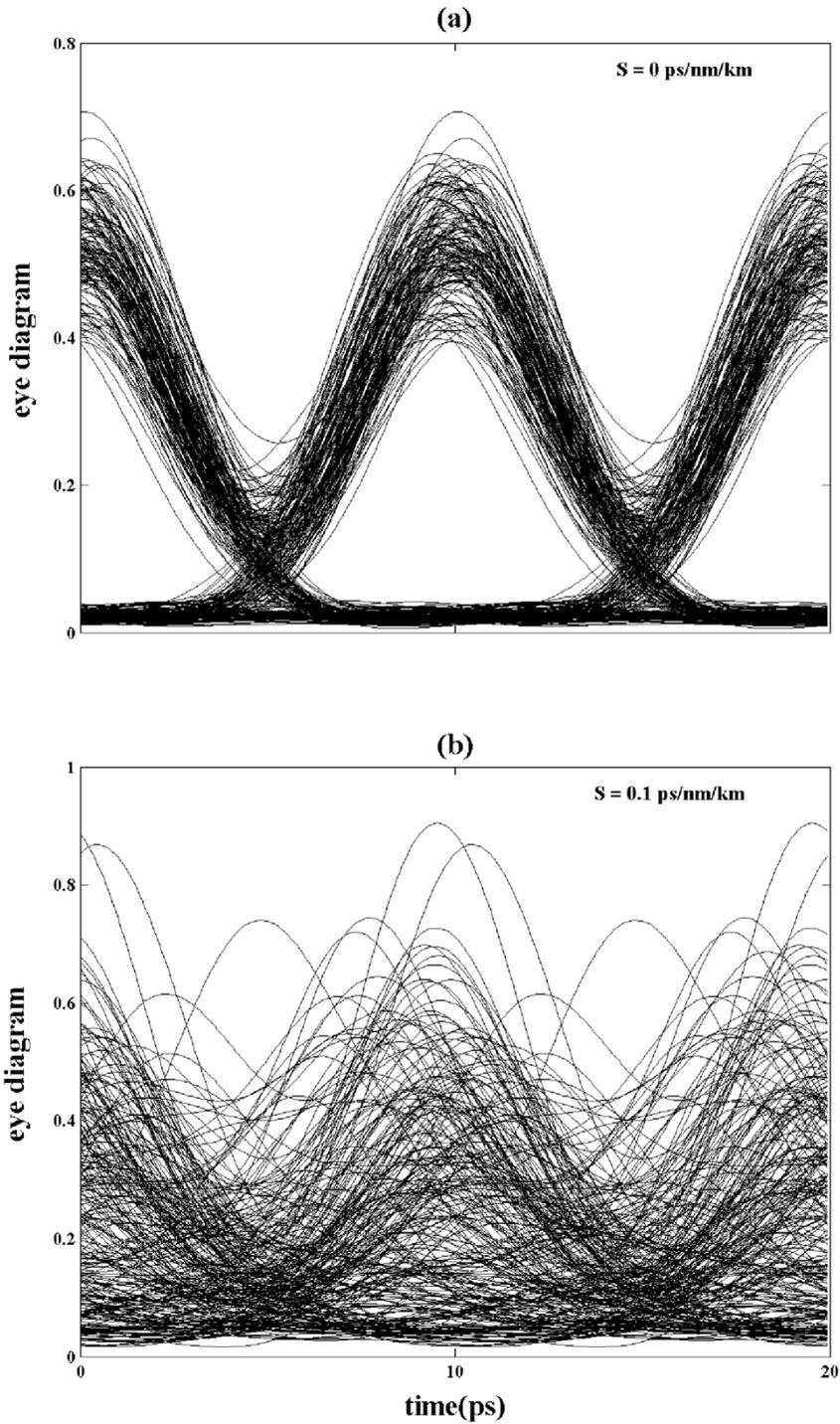
Figure 1. Eye diagram of the electrical signal after propagating 2000 km. In (a) the dispersion slope is considered negligible ( $S=0$  ps/nm<sup>2</sup>/km) and in (b) the dispersion slope coefficient is  $S=0.1$  ps/nm<sup>2</sup>/km. In both cases, five realizations with 64 bits each are represented. The PMD parameter is  $D_p=0.05$  ps/km<sup>1/2</sup>.
