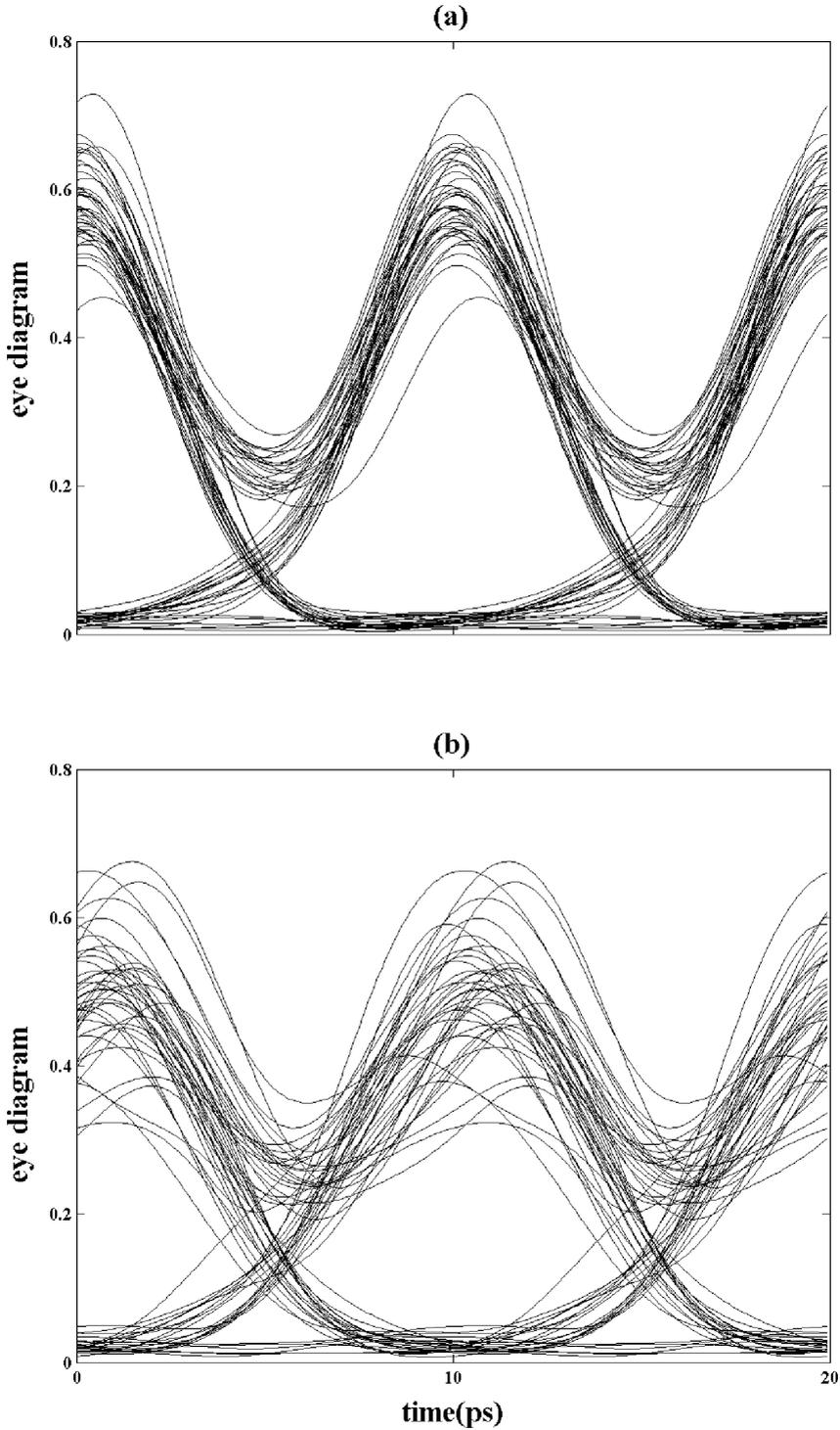
Figure 5. Worst eye diagrams of the electrical signal with slope compensation module with ripple  $A_{\text{GDR}} = 1$  ps and  $1/T_{\text{GDR}} = 200$  GHz: (a) after propagating 1000 km (b) after propagating 2000 km.
