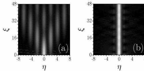
Fig. 2. Beam propagation dynamics in (a) harmonic lattice and (b) lattice with FM rate  $\alpha = 0.11$ . Lattice depth  $p = 3.4$  and frequency  $\Omega = 3$ . Linear medium.
