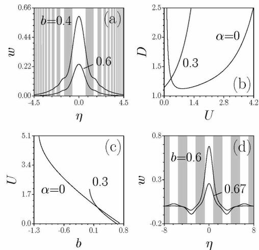
Fig. 4. (a) Profiles of solitons supported by FM lattice at  $\alpha = 0.3$ . (b) Soliton width versus energy flow. (c) Energy flow versus propagation constant. (d) Profiles of solitons supported by harmonic lattice. In all cases  $p = 2$ ,  $\Omega = 2$ . Defocusing medium.
