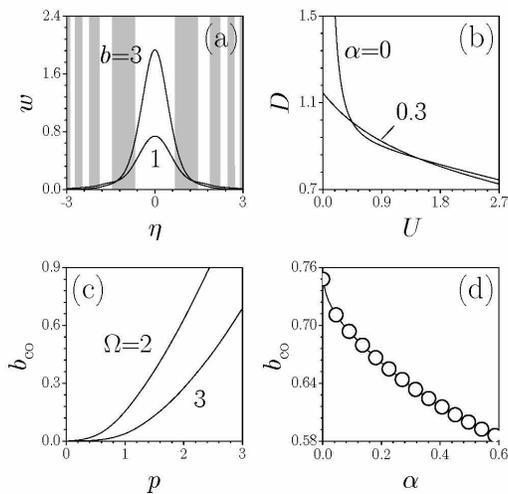
Fig. 3. (a) Profiles of solitons supported by FM lattice at  $p = 2$ ,  $\Omega = 2$ ,  $\alpha = 0.3$ . (b) Soliton width versus energy flow at  $p = 2$ ,  $\Omega = 2$ . (c) Propagation constant cutoff versus lattice depth at  $\alpha = 0.3$ . (d) Propagation constant cutoff versus frequency modulation rate at  $p = 2$ ,  $\Omega = 2$ . Focusing medium.
