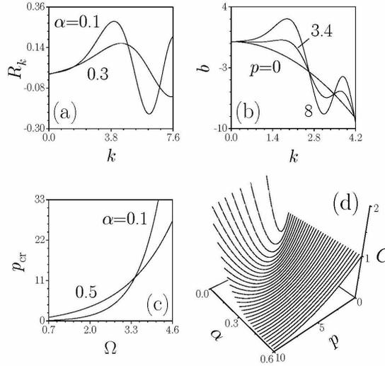
Fig. 1. (a) Spatial spectrum of FM lattice at  $\Omega = 3$ . (b) Dispersion curves at  $\Omega = 3$  and  $\alpha = 0.1$ . (c) Critical lattice depth versus lattice frequency. (d) Integral factor  $C$  on  $(p, \alpha)$  plane at  $\Omega = 3$ .
