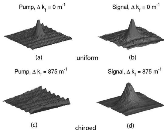
Fig. 2. Engineered solitons. Top row: surface plots show spatial intensity profile of (a) pump and (b) signal components of a multicolor soliton in a uniform grating at  $\Delta k=0$ . Bottom row: surface plots of pump (c) and signal (d) waves at the output of a chirped grating with initial wave-vector mismatch  $\Delta k_i=0$  and final mismatch  $\Delta k_f=875$   $\text{m}^{-1}$ . Note the clearly higher conversion efficiency in the chirped grating case.
