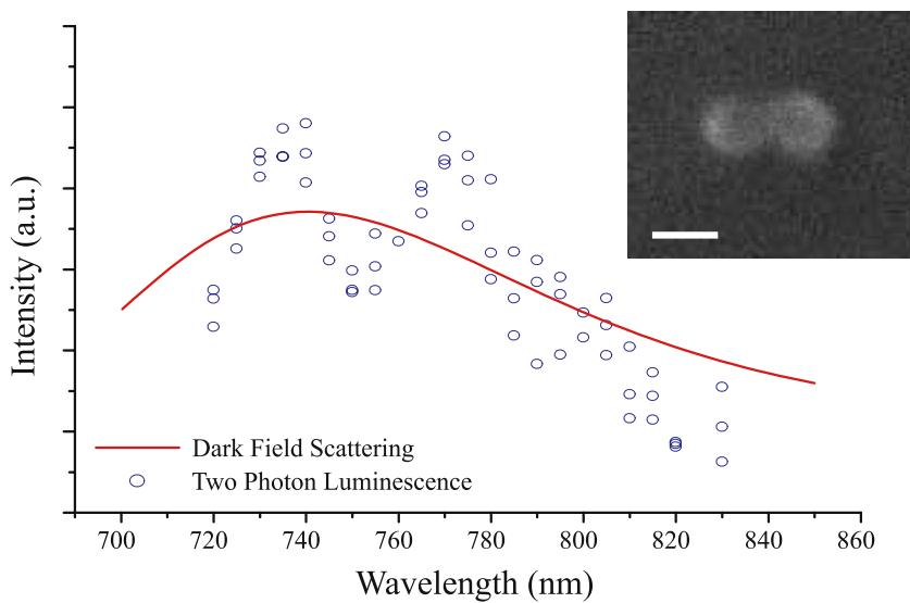
resonance, similar to the scattering one. For the same incident power, the TPL signal in transversal polarization is indistinguishable from the noise level, confirming that our measurement is mainly sensitive to the intense local field in the gap between the two particles.
