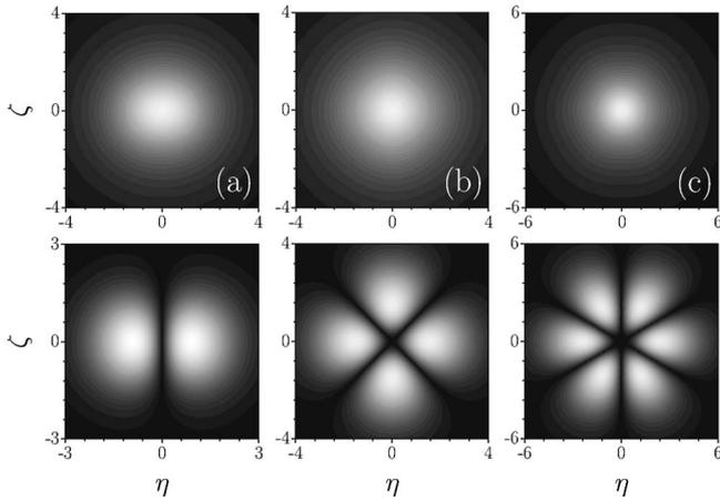
Fig. 1. Total refractive index profile (top row) and field modulus distribution in the second component (bottom) for (a) dipole soliton at  $b_1=3$ ,  $b_2=1.8$ , and  $d=3$ , (b) quadrupole soliton at  $b_1=3$ ,  $b_2=0.9$ , and  $d=4$ , (c) hexapole soliton at  $b_1=3$ ,  $b_2=0.4$ , and  $d=5$ .
