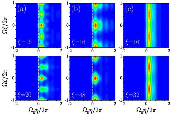
Fig. 4. (Color online) Development of TMI of quasi-1D surface wave at (a)  $\Omega=0.6$ , (b) 1.3, and (c) 1.7. Field modulus distributions are shown at different distances. White dashed lines, interface position. Quasi-1D surface wave corresponds to  $b=5.5$ ,  $E=10$ , and  $p=2$ .
