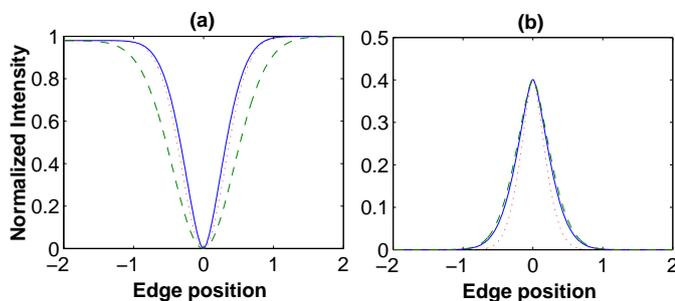
FIG. 2 Numerically calculated values of  $C_m/C_0(\infty)$  (continuous line),  $M_m/M_0(\infty)$  (dashed line) and  $N_m/N_0(\infty)$  (dotted line) when moving the edge of the glass plate (see text for details). The edge position is normalized to the beam width. (a)  $m = 0$ , (b)  $m = 1$ .
