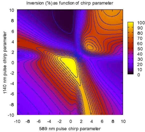
Fig. 3. Final value of the population  $\rho_{22}$  (in %) as a function of the adimensional chirp parameter for the 589 nm ( $a_1$ ) and the 1140 nm ( $a_2$ ) bichromatic pulse components. For instance,  $a_i = 10$  gives a chirp value of  $\approx 0.14 \text{ ps}^{-2}$ . Other parameters are  $t_p = 10 \text{ ps}$ ,  $E_1 = 3.25 \times 10^6 \text{ V/m}$ ,  $E_2 = 4.34 \times 10^6 \text{ V/m}$ ,  $\Delta_1 = 94.14 \text{ GHz}$  and  $\Delta_2 = 10.95 \text{ GHz}$ .
