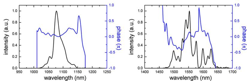
Fig. 2. The retrieved spectral phase and intensity from a FROG measurement of the two arms of an Erbium doped fibre laser. The pulse durations of the 1070 nm arm (left) and 1550 nm arm (right) are 34 and 65 fs respectively. This data is used to create the input pulses for our OPCPA simulation.
