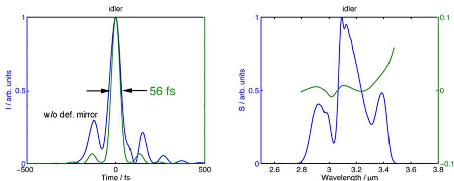
Fig. 5. The left graph shows the pulse in the temporal domain, after compression to 56 fs with (green) the deformable mirror. The blue line shows the 73 fs FWHM compressed pulse without the deformable mirror compensation. The right hand graph shows the spectrum and residual spectral phase that must be corrected by the deformable mirror, which is less than 0.06 radians across the entire spectrum.
