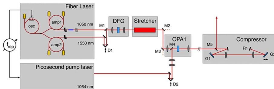
Fig. 1. Mid-IR OPCPA design concept: a commercial fibre laser provides pulses at 1050 and 1550 nm, which are combined through DFG to generate  $3.4\ \mu\text{m}$  radiation (HNLFF - highly non-linear fibre). The mid-IR DFG output is downchirped in a bulk stretcher and amplified in an OPCPA stage, using a commercial 100 kHz Nd:YVO<sub>4</sub> laser as a pump. Finally, the amplified pulse is compressed by a grating compressor (R1 - retro-reflector).
