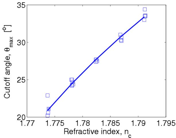
FIG. 4 (color online). Experimental cutoff angle  $\theta_{\max}$ . The results are presented for five different index-matching liquids (squares) together with the theoretical cutoff angle at  $T = 23.0^\circ\text{C}$  (solid line).
