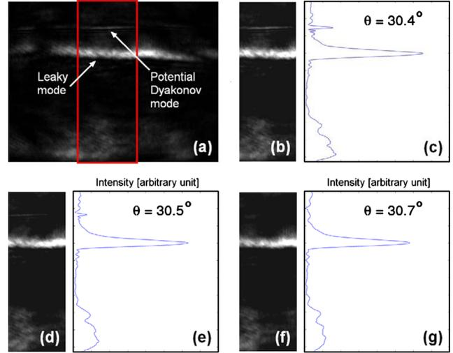
FIG. 3 (color online). Experimental observation for an M1.795 liquid (a) image obtained by CCD camera for  $\theta = 30.4^\circ$ . Dimensions of the image in degrees:  $0.21^\circ \times 0.16^\circ$ . The rectangle indicates the portion of the image shown in (b) at  $\theta = 30.4^\circ$ , (d) at  $\theta = 30.5^\circ$ , and (f) at  $\theta = 30.7^\circ$ . (c), (e), and (g) show the integrated intensity along the lateral direction for images (b), (d), and (f), respectively.
