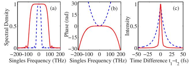
FIG. 4. (Color online) (a) Spectral density  $|\Phi|^2$ , (b) phase  $s_k L/2$ , and (c) correlation time  $|\Psi(t_1-t_2)|^2$  of the biphoton for type-I BBO crystal without tilt (dashed line) and with tilt (solid line). The shrinking of the temporal correlation is clearly observed.
