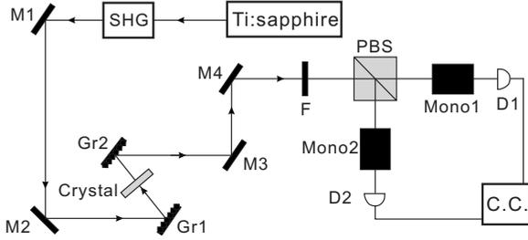
FIG. 1. Experimental setup. SHG: second-harmonic generation; M: mirrors; Gr: gratings; F: long-pass filter; PBS: polarizing beam splitter; Mono: monochromators; D: detectors; and C.C.: coincidence electronics.
