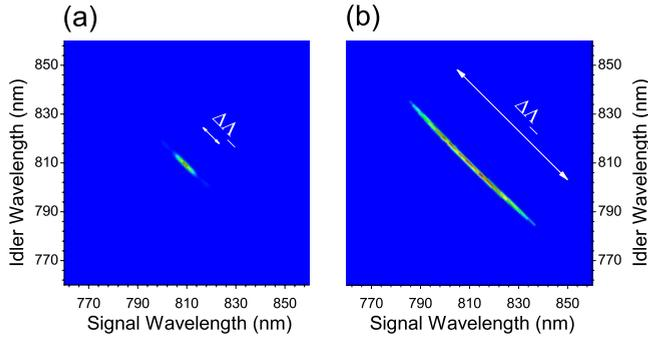
FIG. 2. (Color online) Measured joint spectral density: (a) tilt  $\xi_p=0^\circ$  and (b) tilt  $\xi_p=38^\circ$ . The joint spectrum broadens sevenfold as expected.
