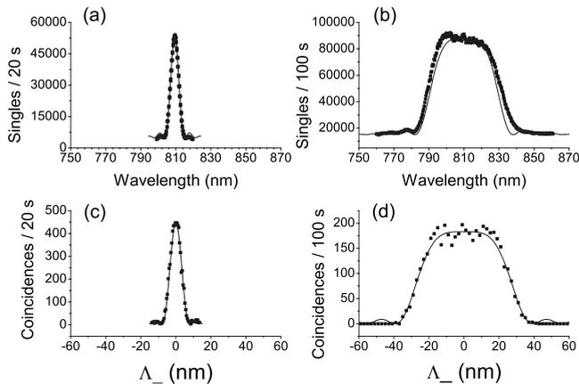
FIG. 3. (a) Signal single counts for  $\xi_p=0^\circ$ ;  $\Delta\lambda_s=5.2$  nm. (b) Signal single counts for  $\xi_p=38^\circ$ ;  $\Delta\lambda_s=41$  nm. (c) Coincidences along the antidiagonal for  $\xi_p=0^\circ$ ;  $\Delta\Lambda_-=7.5$  nm. (d) Coincidences along the antidiagonal for  $\xi_p=38^\circ$ ;  $\Delta\Lambda_-=52$  nm. Solid lines represent the theoretical prediction; squares are the experimental data.
