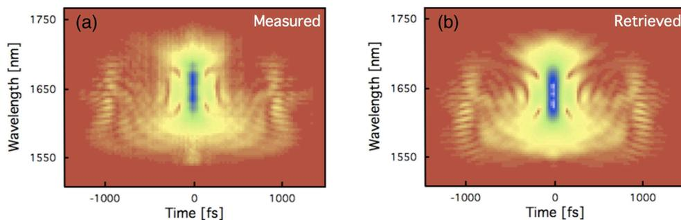
Fig. 3. Measured and retrieved FROG traces. (a) Measured FROG trace of the mid-IR pulse - the colour scale represents the square root of the normalised intensity, chosen to highlight the small features (b) Retrieved FROG trace of the mid-IR pulse, using the same colour scale.
