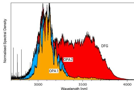
Fig. 2. Spectra at each nonlinear stage. The mid-IR spectrum after the difference frequency generation (red), first (orange) and second (blue) OPCPA stages.
