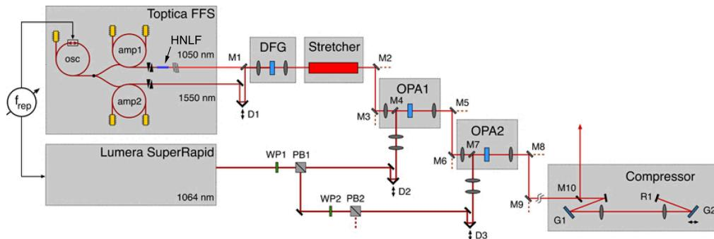
Fig. 1. Mid-IR OPCPA source layout. Two arms of a fibre laser (HNLF = highly nonlinear fibre) are combined through DFG to generate  $3.2 \mu\text{m}$  radiation. This is then amplified by a double stage OPCPA pumped by a Nd:YVO<sub>4</sub> laser and finally compressed by a Martinez-type compressor. WP are waveplates, PB are polarising beamsplitters, D are delay stages, M1,4,7 are dichroic mirrors and other M represent gold mirrors.
