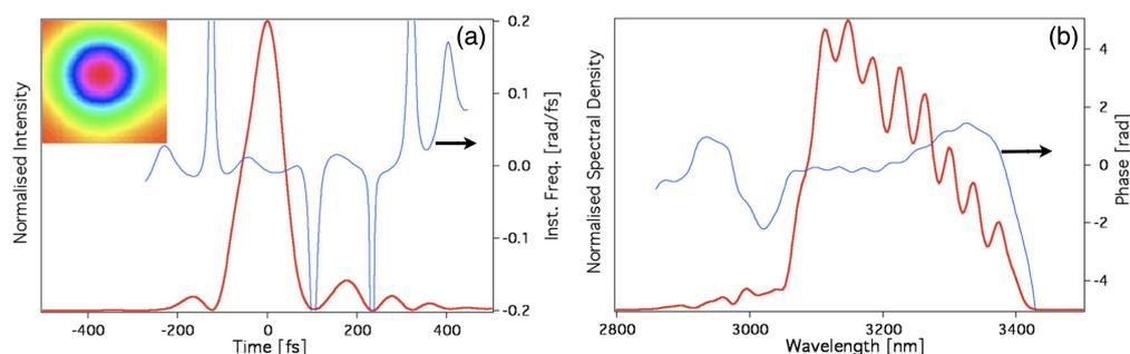
Fig. 4. Reconstructed pulse from the FROG measurement. (a) Temporal profile and instantaneous frequency retrieved by the FROG: 96 fs FWHM = 9.0 cycles (at  $3.2 \mu\text{m}$  one cycle = 10.7 fs) The spatial profile is shown in inset, width of image corresponds to 5 mm (b) Spectrum and phase retrieved by the FROG .
