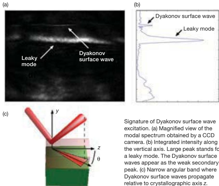
Signature of Dyakonov surface wave excitation. (a) Magnified view of the modal spectrum obtained by a CCD camera. (b) Integrated intensity along the vertical axis. Large peak stands for a leaky mode. The Dyakonov surface waves appear as the weak secondary peak. (c) Narrow angular band where Dyakonov surface waves propagate relative to crystallographic axis  $z$ .
