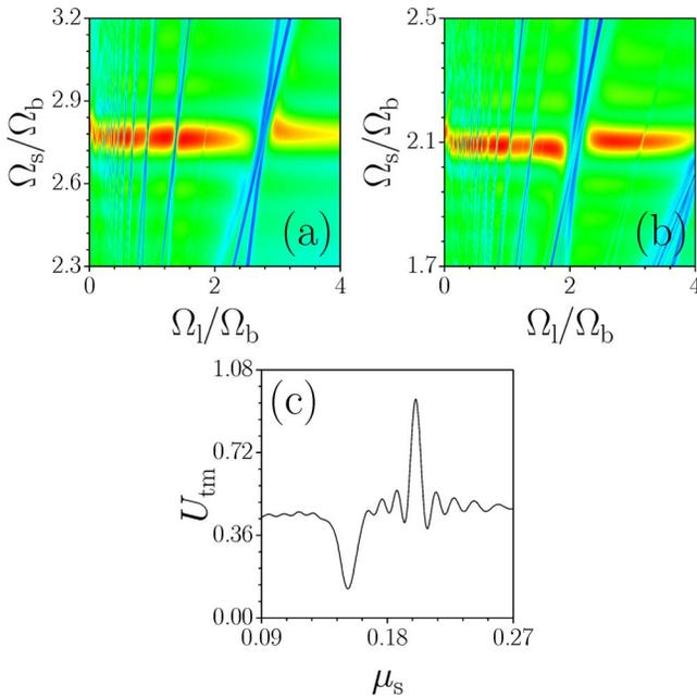
Fig. 3. (Color online) The product of distance-averaged energy flows  $U_{tm}=U_{1m}U_{2m}$  versus modulation frequencies  $\Omega_s$  and  $\Omega_l$  at (a)  $\mu_s=0.20, \mu_l=0.10$  and (b)  $\mu_s=0.15, \mu_l=0.15$ . Red regions correspond to strongest inhibition of tunneling when  $U_{tm}\approx 1$ , while in blue regions one has strongest delocalization when  $U_{tm}\rightarrow 0$ . (c)  $U_{tm}$  versus  $\mu_s$  at  $\mu_l=0.1, \Omega_s=2.77\Omega_b, \Omega_l=1.23\Omega_b$ .
