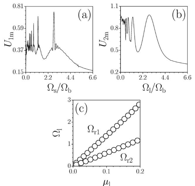
Fig. 2. (a) Distance-averaged energy flow in the input channel versus  $\Omega_s$  at  $\mu_s=0.2$ ,  $\mu_l=0$ . (b) Distance-averaged energy flow in the input coupler versus  $\Omega_l$  at  $\mu_s=0$ ,  $\mu_l=0.2$ . (c) Frequencies of first and second resonances versus  $\mu_l$  for  $\mu_s=0$ .
